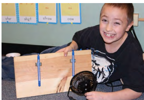
Figure 2. An enthusiastic student making wet and dry bulb temperature measurements during the weather club.
