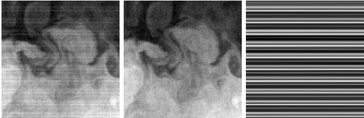
Figure 1. (left) Original image from Terra MODIS band 20 affected with stripe noise (middle) Image processed with the UVDM (right) Extracted stripe noise showing, as expected, strong anisotropic characteristics.
