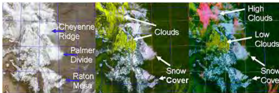
Figure 3. Comparison between True Color (left), the binary Cloud /Snow Discriminator product (middle), and the Cloud Layers & Snow Cover Discriminator product (right) imagery over the north-central United States as collected by NASA's MODerate-resolution Imaging Spectroradiometer (MODIS) sensor. In the Cloud Layers & Snow Cover product, white areas denote snow cover, yellow areas denote low cloud cover (liquid), orange/magenta areas denote high cloud cover (mixed/ice), and green areas denote clear sky surface.
