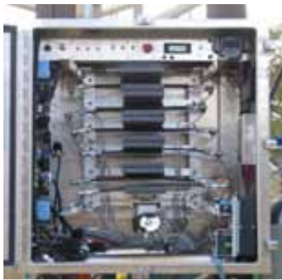
Figure 8. Precision carbon dioxide and flask sampling system (left) and midday atmospheric CO 2 concentration measurements (right) at the Skukuza eddy flux site in the Kruger National Park, South Africa. The system uses automatic calibration with WMO-traceable standards and a temperature controlled infrared gas analyzer to measure CO 2 concentration to an absolute precision of ~0.2 ppm.
