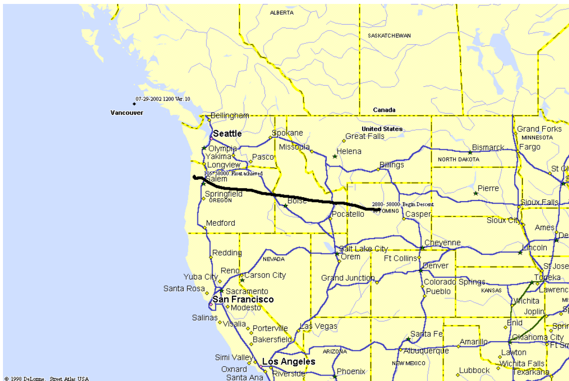
Figure 1. Trajectory predicted for a balloon launched at 1200 UTC 29 July 2002 from Tillamook, Oregon based upon global Aviation model winds. Float altitude is 58,000 ft; ascent and descent rates are 500 fpm and 600 fpm, respectively.
