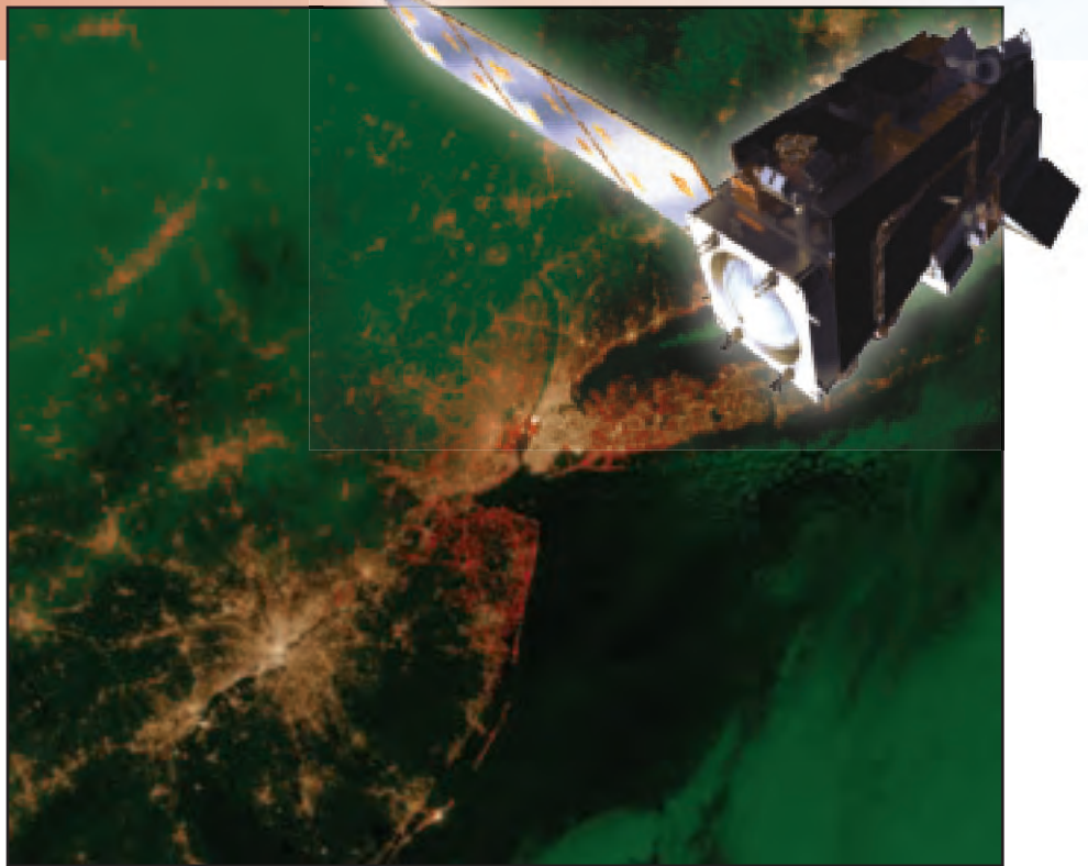
Figure 3. Composite image of nighttime light sources over metropolitan New York, comparing light sources between 25 September and 1 November, 2012, as seen by the day-night band sensor aboard Suomi NPP. Red pixels denote areas without power after the passing of Hurricane Sandy on the 29th of October 2012.
