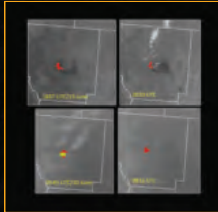
Figure 4. Series of MODIS images from 19 and 20 June outline the actively burning area of High Park Fire. Red pixels denote locations with a high probability of fire, while yellow pixels denote a high probability of very hot fire activity. MODIS-derived fire detection algorithms are used to locate active fires in remote areas and track movement of known fires. Credit: Steve Miller/CIRA
