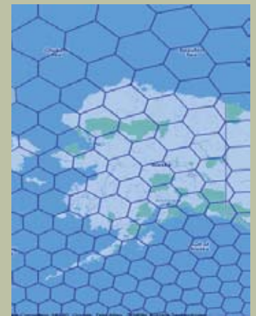
Figure 4: A portion of the FIM grid displayed in Google Maps, from roughly the 50th to the 75th parallel. Notice the shape distortion (of the otherwise area-equivalent icosahedral grid cells) increases towards the upper latitudes.
