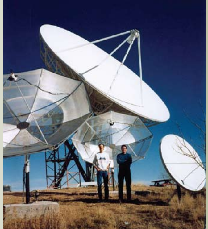
Figure 1. Some of the antennas used to collect GOES data for ISCCP. The 10-meter dish in back was the first antenna. In the foreground are engineers Michael Hiatt and Duane Whitcomb. Photo taken ca. 1995.
