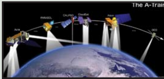
Figure 3. “A-Train” satellite constellation. The lead satellite in the A-Train is the NASA EOS Aqua. The other A-Train satellites that follow are CloudSat, a NASA-CNES lidar satellite (CALIPSO), a CNES satellite carrying a polarimeter (PARASOL), and the NASA EOS Aura.
