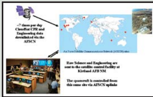
Figure 4. CloudSat data flow – satellite to USAF site at Kirtland AFB.
