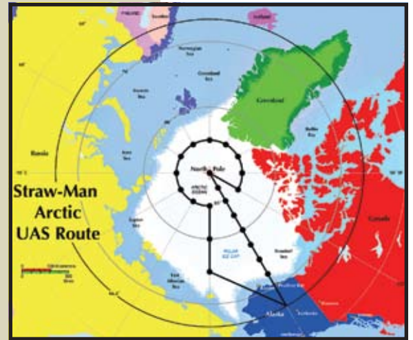
Figure 3. Straw-man Arctic testbed flight path for a long-endurance UAS. Observations such as dropsondes are taken at the locations indicated by black circles along the path.
