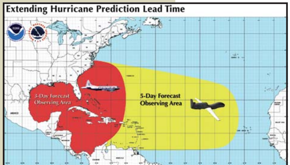
Figure 4. HALE UAS platforms could extend tropical cyclone monitoring across the central Atlantic to observe cyclogenesis and improve forecasting.
