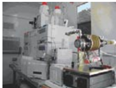
Figure 2 a, the PILS instrument and; b, an 8-week trace of 15 min PILS data collected at Yosemite National Park illustrating the anion components of the fine aerosol.
