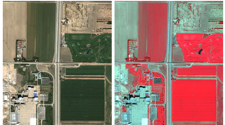
Figure 2. Example of high resolution remote-sensing images acquired from Quickbird™ satellite on Sept 14, 2002 for north of Fort Collins, CO. On the left is the natural color image and on the right is the Color Infrared image. (Image Courtesy: Digital Globe, Inc.) Areas in red suggest high quantity of healthy green vegetation.
