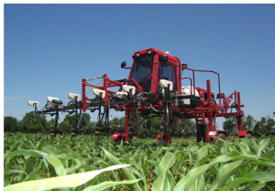
Figure 3. Asuite of active remote-sensing devices mounted on a high-clearance tractor, eq uipped with variable rate fertilizer controller in the back. [Photo courtesy: Oklahoma State University.
