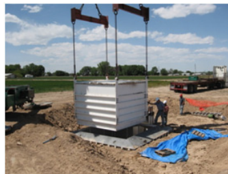
Figure 2. The inner tank plus soil being lowered inside the containment tank of the crop lysimeter. Photo taken by Michael Bartolo.
