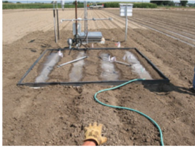
Figure 8: Water being applied to the soil monolith of the crop lysimeter. Photo taken by Michael Bartolo (CSU-AVRC).
