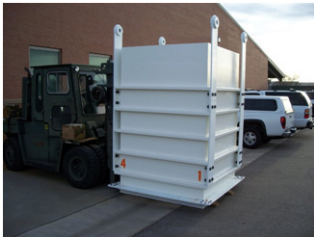
Figure 5. The inner tank of the reference lysimeter, set on a forklift. The four outer bars were temporarily attached for lifting and lowering of the inner tank during installation. Photo taken by Dale Straw of DWR.
