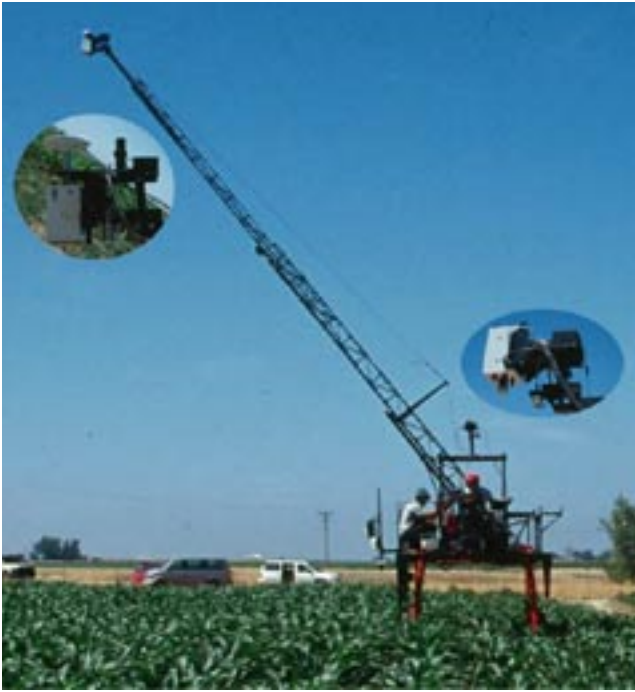
Figure 4. High-clearance tractor instrumented with various remote sensing instrumentation.
