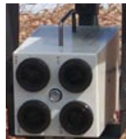
Figure 3. Four channel radiometer manufactured by Exotech Incorporated.
