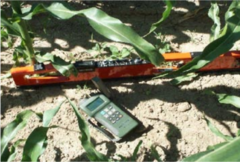
EM-38 quickly measures conductivity in soil.
