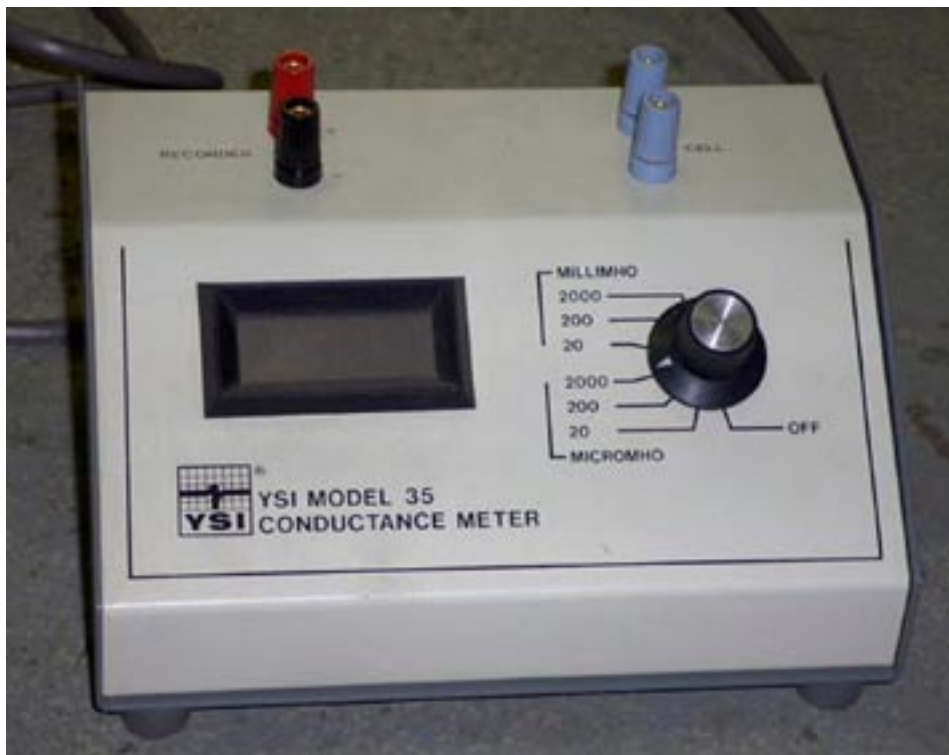
A conductivity meter is used to take an soil EC reading.
