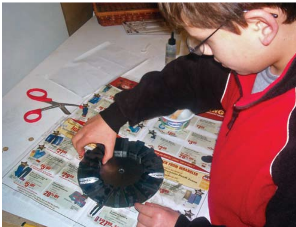
John carefully positions the magnets on a disk that will generate an electrical charge, which is then stored in batteries. He uses the batteries for his other projects and estimates it will take 100 recharges to recover the cost of materials.
