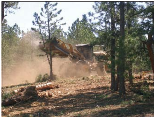
Mechanical fuel reduction often is accomplished by hydro-axe.
