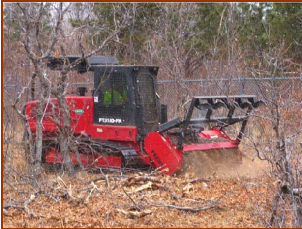
Fuels mitigation at the Cheyenne Mountain Zoo using mastication equipment.
