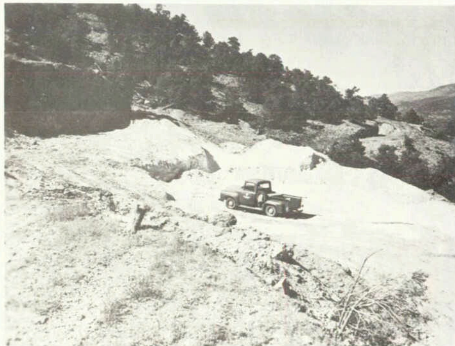
Photo 2--Developed clay deposit (S-49) near Howard, Colorado. Clay deposit has been stripped of overburden so that air-drying of clay can take place. In-place moisture content of clay or bentonite deposits has ranged as high as 50 percent; by air-drying in the pit this can be reduced to 15 to 30 percent.
