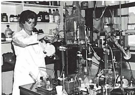
Laboratory technician determining inorganic nitrogen content of the soil samples, San Luis Valley Branch Experiment Station, Center, Colorado.
