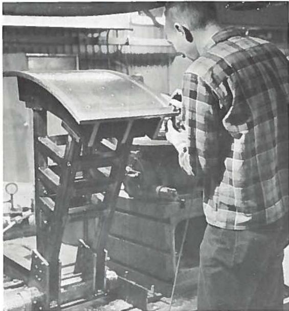
**Model of radial gate used in the Tarbela Dam.**
