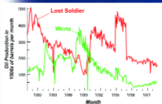
Figure 2 Oil production histories for the two fields at Baroil in Wyoming. Note the three-fold increase in output at Wertz after commencement of CO 2 -EOR in 1987 and an equivalent increase at Lost Soldier in 1989-90.
