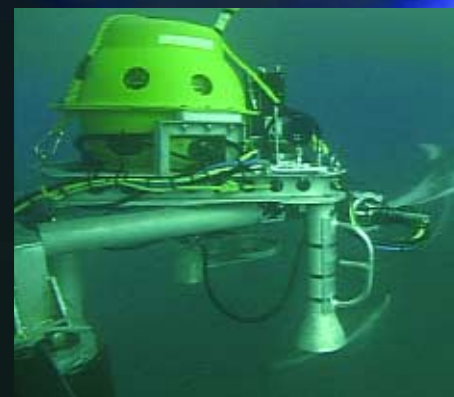
The Raman spectrometer was deployed on the ROV Tiburon.
