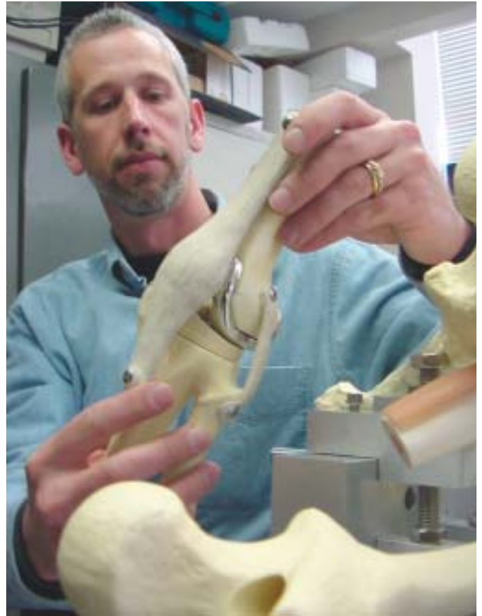
Bach applies stresses to the knee to determine how knee ligament injuries occur and how to prevent them.
