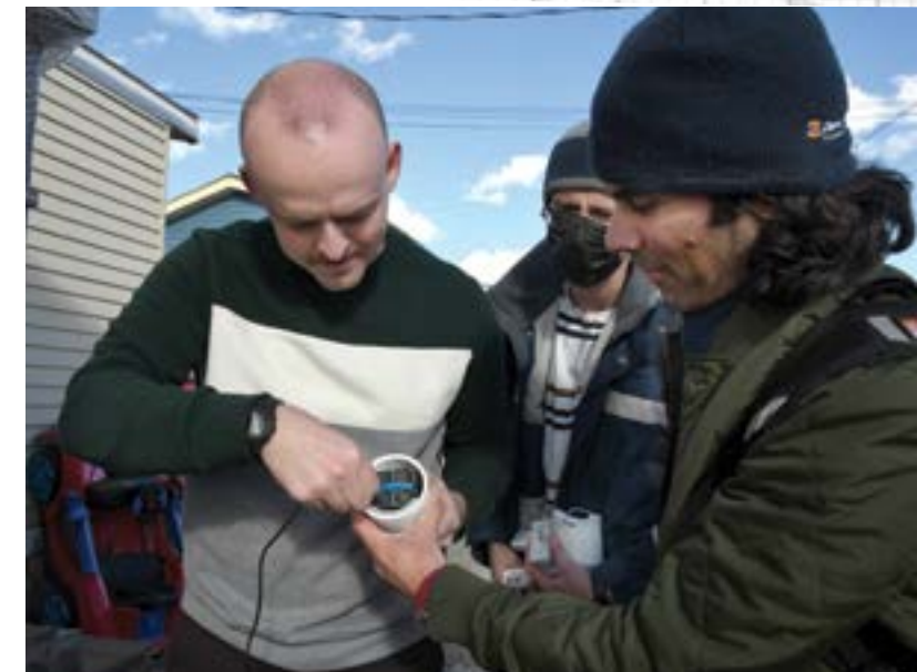
Graduate students Karlyle Munz and Daniel Safronov and Associate Professor Paulo Tabares-Velasco install an outdoor particulate matter (PM 2.5 ) sensor in a low-income neighborhood in Colorado to compare indoor and outdoor PM 2.5 concentrations and measure air temperature.
