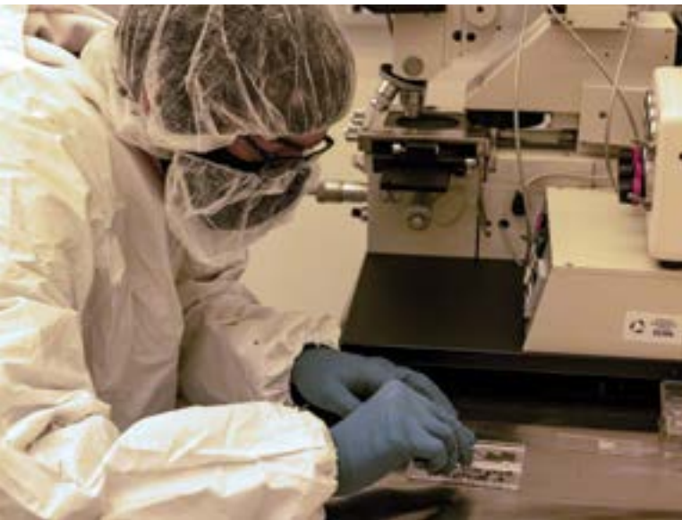
Graduate student Matt Tennerly prepares a silicon sample for photolithography in the clean room on campus.
