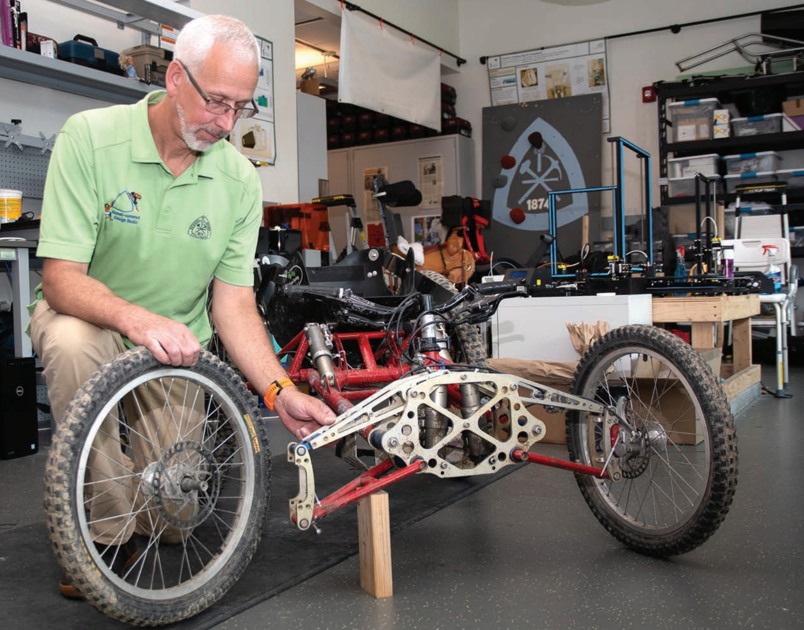
The Human Centered Design Studio works like a design firm, with students working on multiple client-driven projects, including a four-wheel mountain bike (above), a cross-country sit ski and more.
