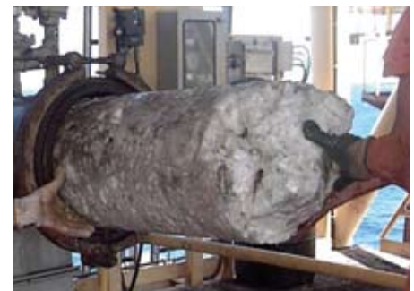
Clockwise from Top: A precisely modulated downward current in CSM's DOGWB simulator prototype keeps a gas bubble stationary. By varying temperature, pressure and chemical composition, researchers are able to observe phenomena such as oil/gas dispersion in water and the formation of gas hydrates, such as those encountered in an oil/gas well blowout; a hydrate plug is removed from a pipeline; hydrate encrusted gas bubbles form in a high pressure water column, leading to blockage of the channel; illustrations of containment and response in the Macondo well.
