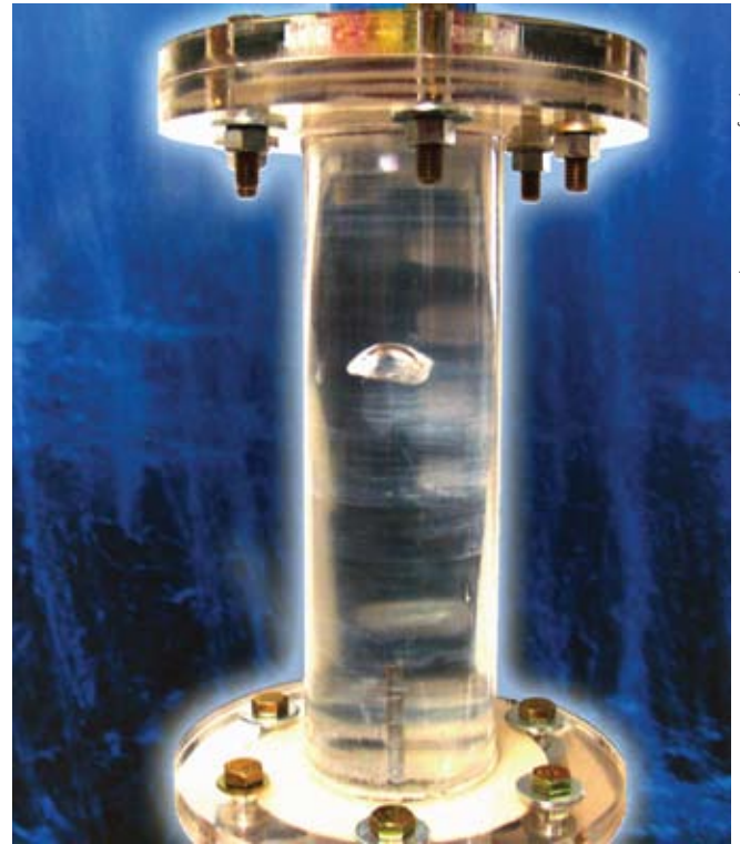
Clockwise from Top: A precisely modulated downward current in CSM's DOGWB simulator prototype keeps a gas bubble stationary. By varying temperature, pressure and chemical composition, researchers are able to observe phenomena such as oil/gas dispersion in water and the formation of gas hydrates, such as those encountered in an oil/gas well blowout; a hydrate plug is removed from a pipeline; hydrate encrusted gas bubbles form in a high pressure water column, leading to blockage of the channel; illustrations of containment and response in the Macondo well.
