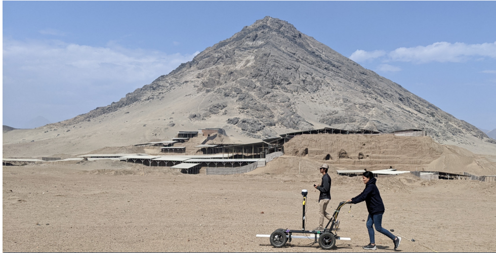
Jared Low is working with UNSA student Merianth Verástegui Marín to gather frequency-domain electromagnetic data at the Huacas de Moche archaeological site in Trujillo, Peru. Specifically, data are being collected above an extensive Moche residential center between the temple Huaca de la Luna and the ancient palace known as Huaca del Sol, the two major pyramids at the site. In the background of the photo are Cerro Blanco (the mountain) and the temple Huaca de la Luna. (Photo: Richard Krahenbuhl)
