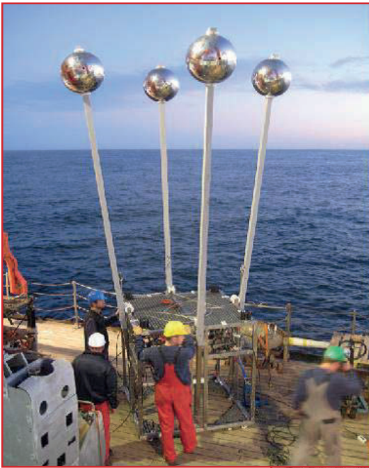
Right: An electromagnetic receiver that measures the two horizontal components of the electric field on the seafloor
