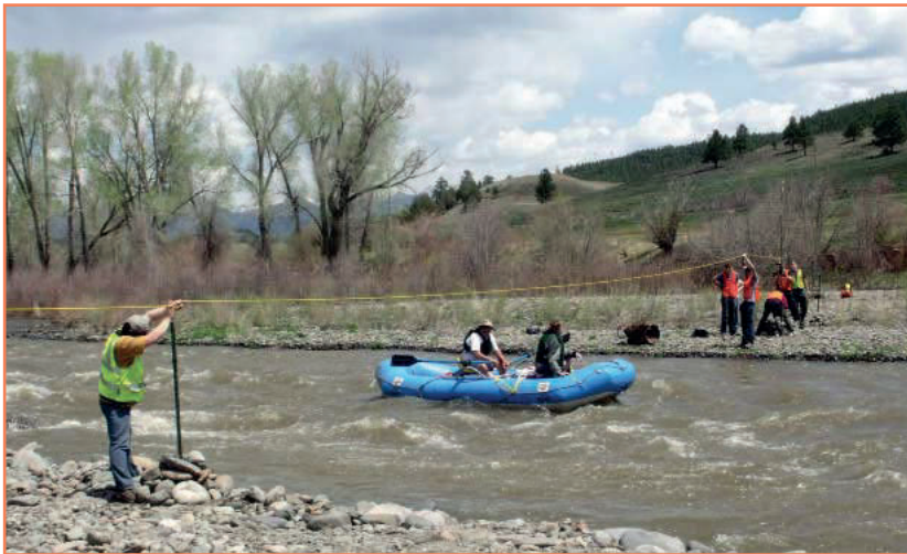
Stringing DC resistivity cable across the San Juan River near Pagosa Springs, Colorado
