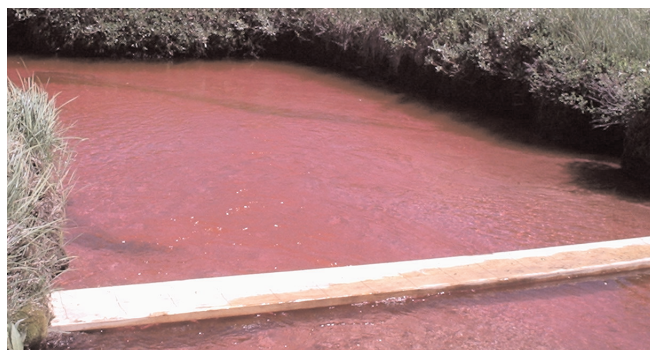
The results of rhodamine and salt used for the stream tracer.
