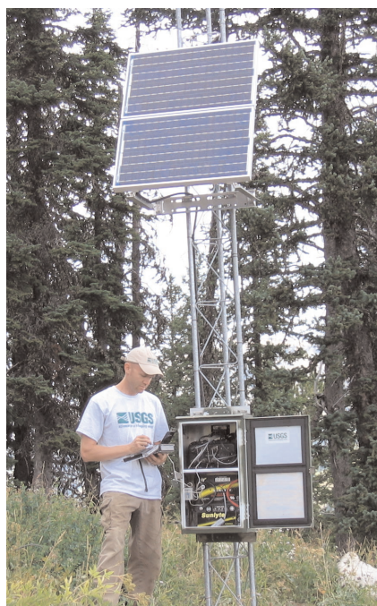
Checking data flow and the health of a station via a palm-pilot at station TPAW, up on Teton Pass.
