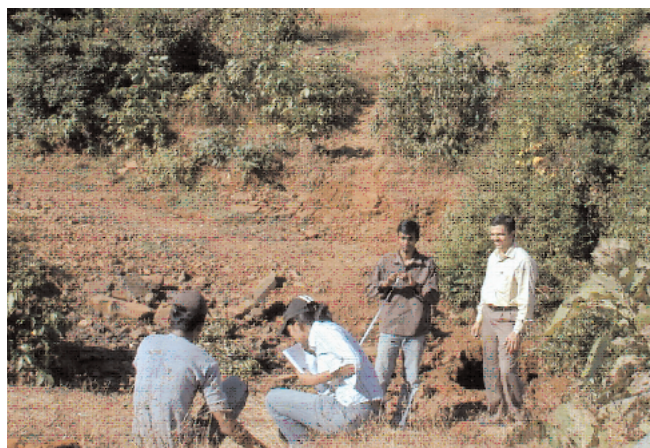
In the valley proposed for the dam, students map the catchment area and make pits to assess subsurface lithology.
