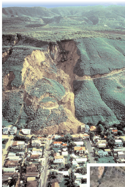
La Conchita, California Landslides of 1995 (left) and 2005 (below) caused by massive rain storms.
