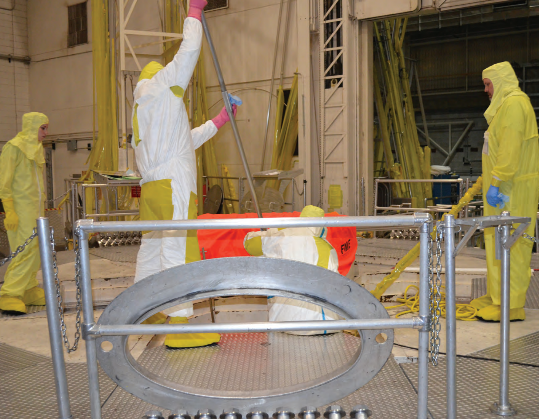
Technicians at Idaho National Laboratory insert Mines' experiment, comprising 288 samples of stainless steel and Inconel alloys, into the Advanced Test Reactor.
