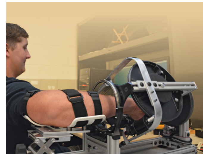
Mechanical engineering student David Long demonstrates how to perform exercises using the Wrist Gimbal.
