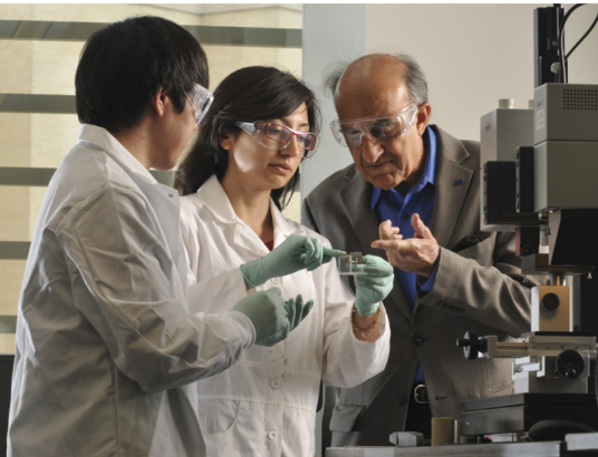
From left, graduate students Younki Cho, Somayeh Karimi and Professor Hossein Kazemi examine a Drop Shape Analyzer (DSA 100) chamber (top photo) to determine the contact angle between oil and a shale sample in the brine-oil environment.
