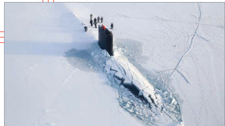
The Los Angeles-class attack submarine USS Hampton breaks thin ice to surface in the Arctic Ocean during the 2014 ICEX campaign.
