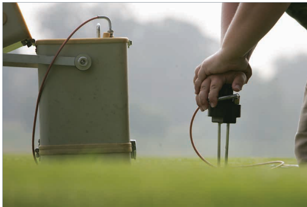
Marisa Griffin, agriculture research coordinator in crop and soil science uses a device (TDR) to measure moisture in the turf at the UGA College of Agriculture in Griffin, Ga. Credit: John Amis
