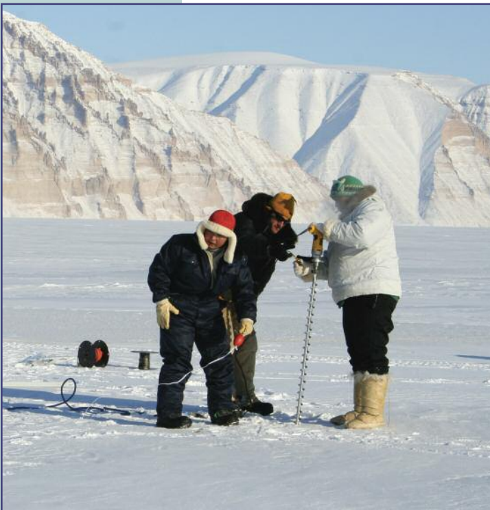
Toku Oshima and Mamarut Kristiansen, hunters from Qaanaaq, Greenland, work with Andy Mahoney to install a sea ice-monitoring station near their community. (Courtesy Shari Gearheard)
