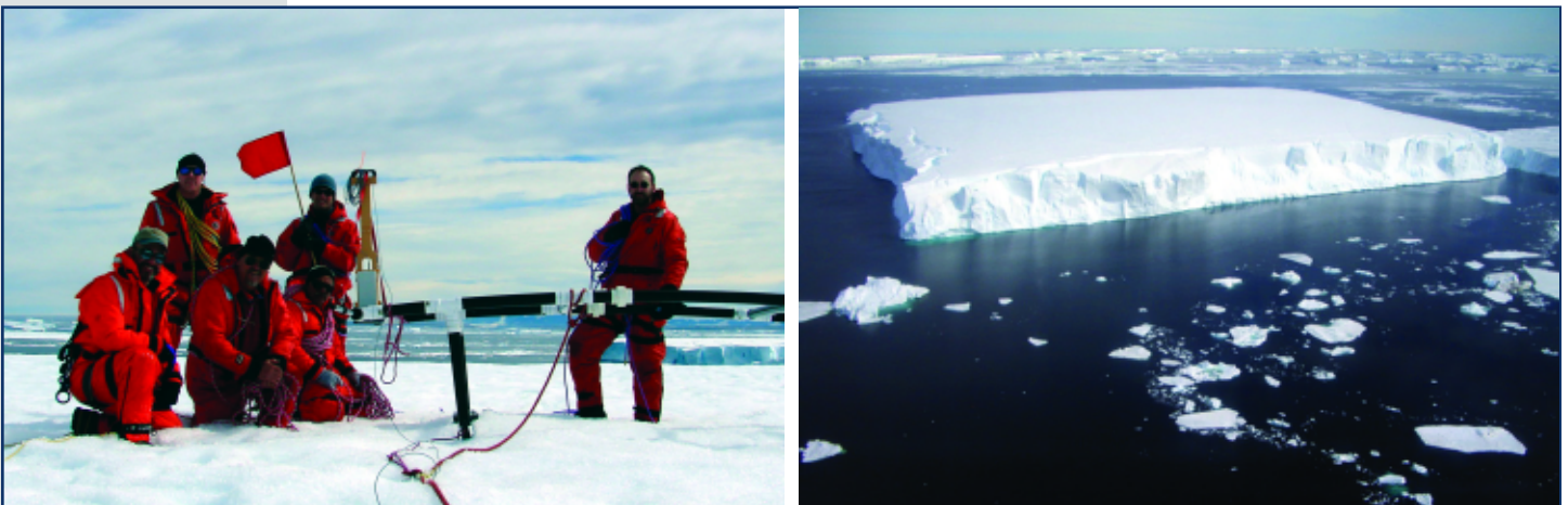
The IceTrek team tests setting up the 25-Mhz radar instrument (left) on a small Antarctic iceberg, nicknamed “Chip” (right), before installing their equipment on the larger AMIGOSberg and A22A icebergs. (Courtesy Ted Scambos, NSIDC)
