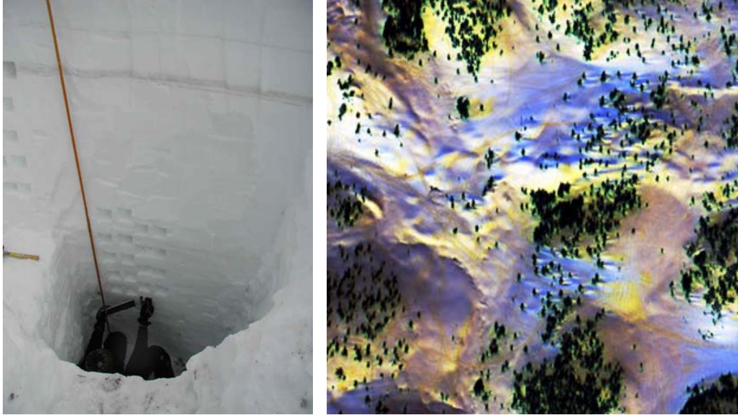
Figure 3: Former NSIDC employee, Kate Daniels, takes a snow density sample at the bottom of a deep snow pit near Rabbit Ears Pass, Colorado (left). Hyperspectral image of the Walton Creek Intensive Study Area in the Rabbit Ears Meso-cell Study Area, acquired March 31, 2003, by the NASA/JPL Airborne Visible Infrared Imaging Spectrometer (AVIRIS). The image shows an area of 1 km 2 and has a spatial resolution of ~ 2 m. The snow cover and grain size were generated with the Multiple Endmember Snow Covered Area and Grain-size model. This and other such images will be used for validating snow cover retrievals from the microwave data collected during the CLPX, and in forward modeling the passive microwave emission from snow-covered forested terrain.
