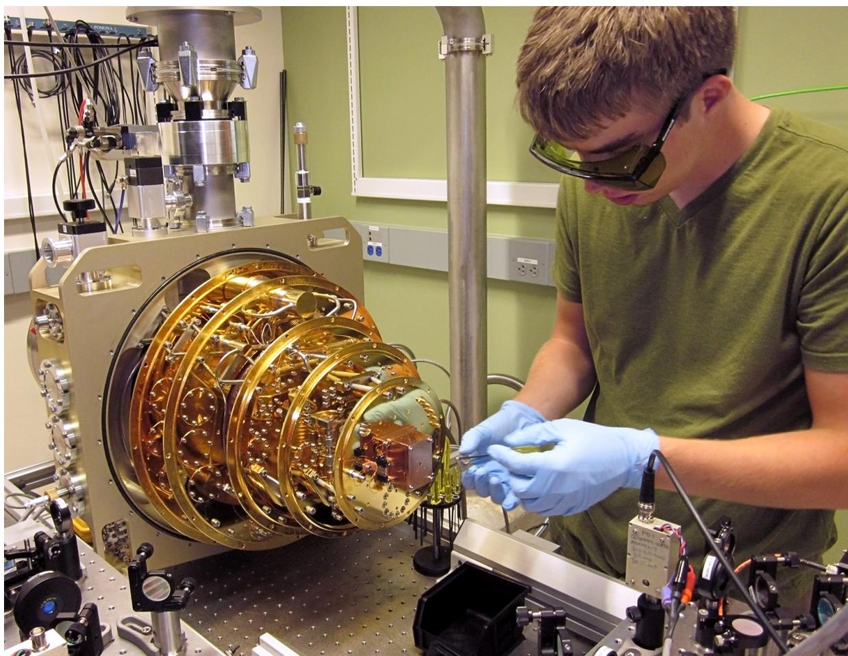
To investigate how cold a tiny drum could get if it were laser cooled down to a limit set by the laws of quantum mechanics, graduate student Bob Peterson (shown here) and his colleagues in the Lehnert-Regal lab used this brand new refrigerator featuring gold plating on copper plates. The device can cool down to as low as 30 mK. Laser cooling then further cools a tiny drum to 14  $\mu$ K, more than 2,000 times colder. Credit: The Regal group and Tom Purdy, JILA
