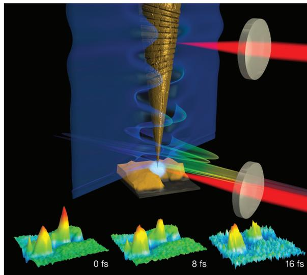
The Raschke group’s novel, ultrafast optical nanoscope is capable of focusing extremely short light pulses to image the behavior of electrons in real space and time on a thin gold film. Because the nanoscope can measure time in femtoseconds and length in nanometers, it may be used in studies of photosynthesis as well as solar cells and other energy conversion and storage materials. Credit: The Raschke group and Steve Burrows, JILA
