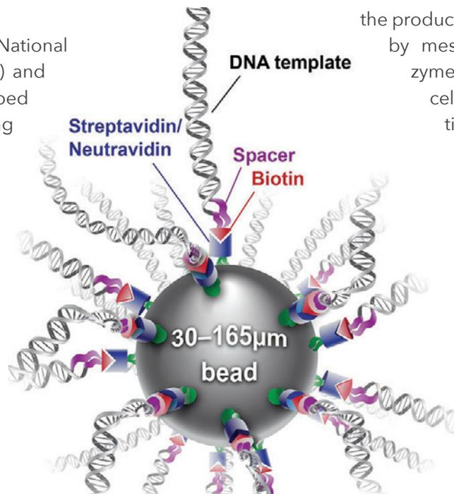
DNA templates made for custom-building RNA strands developed by National Institutes of Health researchers. The custom-built DNA templates are attached to polymer beads. Special enzymes called RNA polymerases use these DNA templates to produce custom-made RNA. Credit: Joseph Meyer, Scientific Publications, Graphics & Media, Leidos Biomedical Research, Inc.
