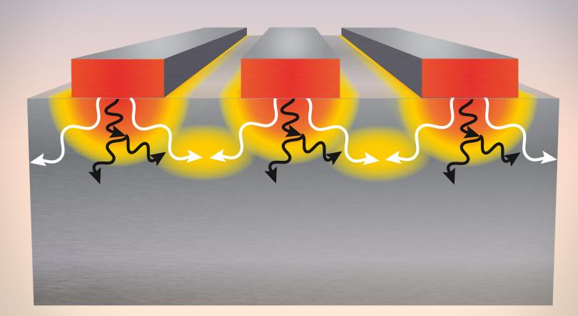
When closely spaced heated nickel nanowires emit lattice vibrations known as phonons into underlying materials, the phonons efficiently collide and transport heat away. This discovery has immediate application to the design of integrated circuits, nanoenhanced solar cells, and other electronics employing nanostructures. Credit: K. Hoogeboom-Pot and the Kapteyn/Murnane group, JILA
