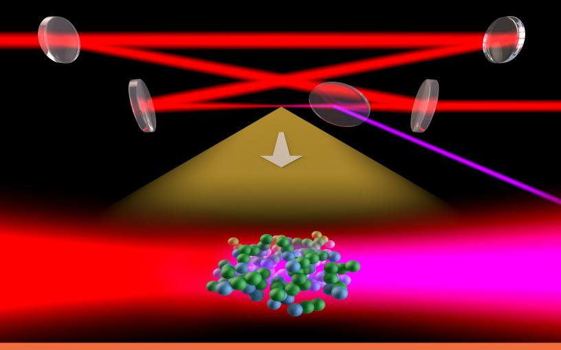
A pulse from a powerful laser can align stick-shaped molecules of laughing gas (N<sub>2</sub>O) inside an optical cavity up to 100 million times a second. A second laser pulse can then initiate high-harmonic generation, a process that occurs when laser-stimulated atoms or molecules emit light of higher harmonics of the fundamental frequency of the laser. Credit: The Ye group and Steve Burrows, JILA
