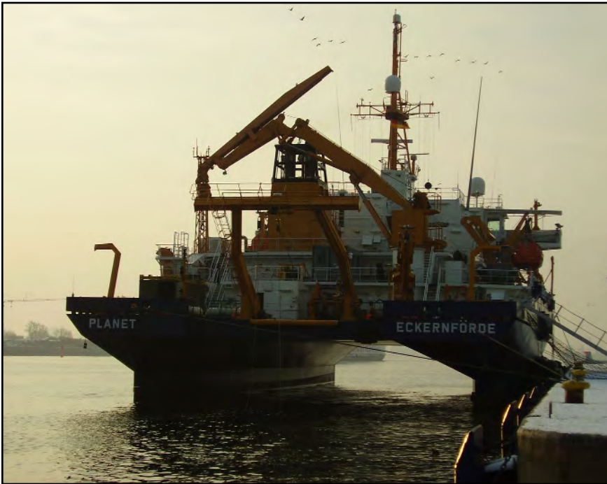
Stern view of FS Planet , a twin-hulled semisubmersible vessel, Baltic Sea, February 2006. Chris Jenkins (INSTAAR) was taking part in engineering tests for the German Navy and U.S. Office of Naval Research to help calibrate models of how dropped objects bury themselves into soft sea-floors. These models will help locate the thousands of mines still buried in the Baltic Sea from the World Wars as well as future port security. Photo: Chris Jenkins (INSTAAR).
