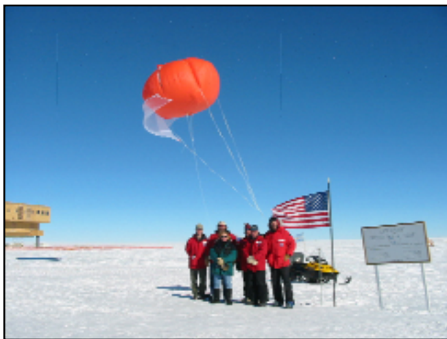
Antarctic Tropospheric Chemistry Investigation (ANTCI) scientists (including INSTAAR's Detlev Helmig) with one of their tethered helium balloons used to study atmospheric transport and chemistry, South Pole, Antarctica, December 2003. The INSTAAR Atmospheric Research Lab is participating in ANTCI. Photo: D. Helmig (INSTAAR).
