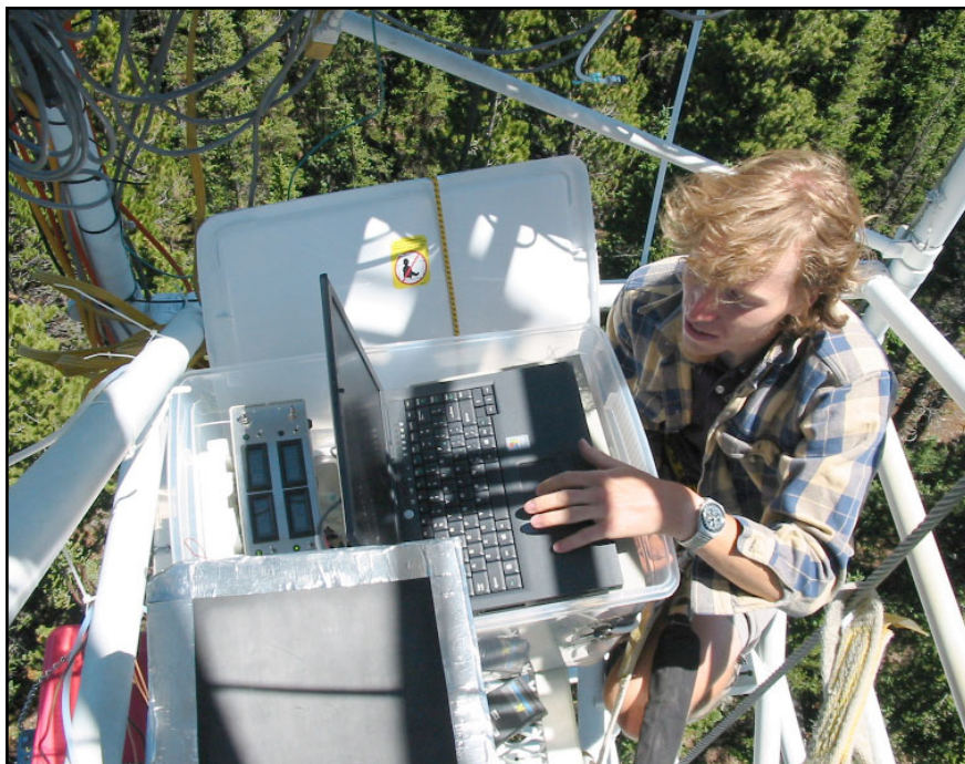
Jacques Hueber (visiting engineering student from France) develops a chemiluminescence ozone analyzer for the measurement of ozone deposition fluxes to the forest at the Niwot Ridge Ameriflux tower, Mountain Research Station, Colorado, August 2002. Photo: D. Helmig
