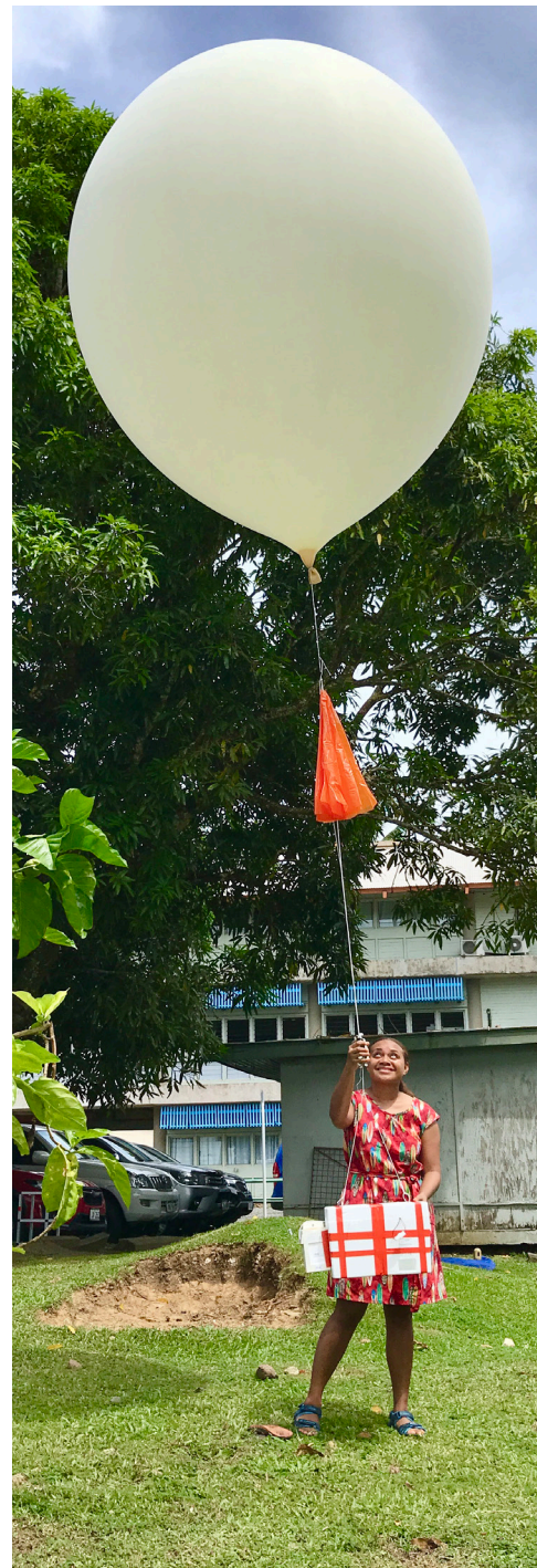
A graduate student at the University of the South Pacific in Fiji launches a weather balloon carrying an instrument to measure ozone. CIRES scientists were critical in helping NOAA measure stratospheric ozone and surface ozone at 17 locations around the world. Photo: Irina Petropavlovskikh/CIRES
