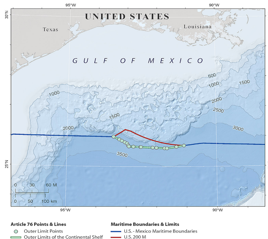
NCEI-13: Map showing the outer limits of the U.S. continental shelf in the Western Gulf of Mexico region. The 16 points connected by straight lines that comprise the outer limit line are the same as those that form the line of delimitation agreed between the United States and Mexico in the June 9, 2000 treaty. Image: NOAA
