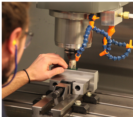
Danny Warren setting up a Computer Numerically Controlled (CNC) milling machine. Photo: Robin Strelow/CIRES
