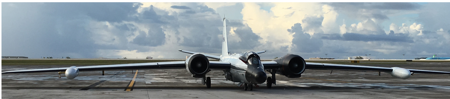
CSD-07: NASA WB-57F high-altitude research aircraft in Guam after completing the first science flight of the Pacific Oxidants, Sulfur, Ice, Dehydration and Convection mission on October 12, 2016. CIRES scientists in NOAA's Chemical Sciences Division operated four of the 11 instruments in the payload. Photo: Troy Thornberry/CIRES and NOAA
