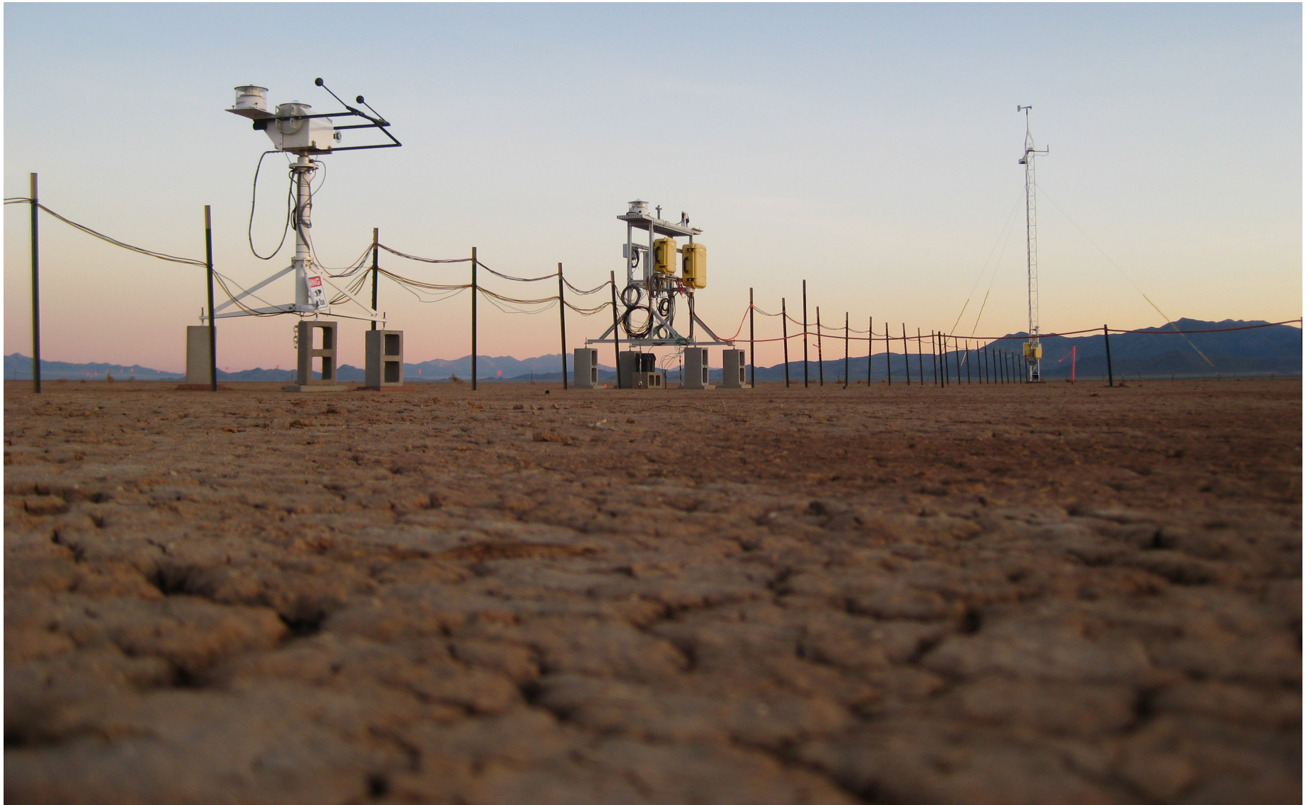
GMD-01: Mobile surface radiation (SURFRAD) site operated by NOAA's Global Monitoring Division Radiation Group located on the dry bed of northern Arizona's Red Lake. Instrumentation is measuring the surface radiation budget. Photo: Gary Hodges/CIRES and NOAA
