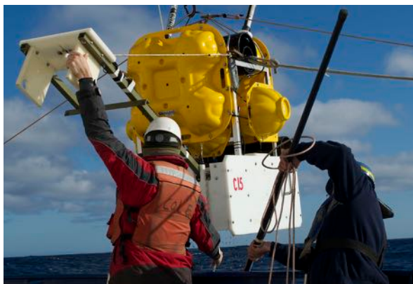
Recovery of Lamont ocean bottom seismometer and absolute pressure gauge package after one year on the seafloor offshore Gisborne, New Zealand. Photo: Elizabeth Brenner/Scripps Institution of Oceanography
