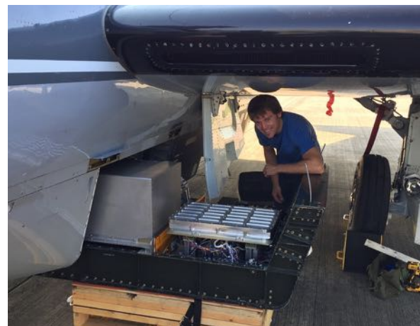
Andrew Rollins installs an SO 2 instrument on a NASA high-altitude research aircraft, preparing for the start of a field experiment based in Houston. Photo: R. Gao/NOAA
