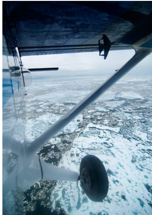
NOAA Twin Otter airplane, with the downward-looking oceanographic lidar onboard, to study plankton layers in the Beaufort Sea north of Barrow, Alaska.
