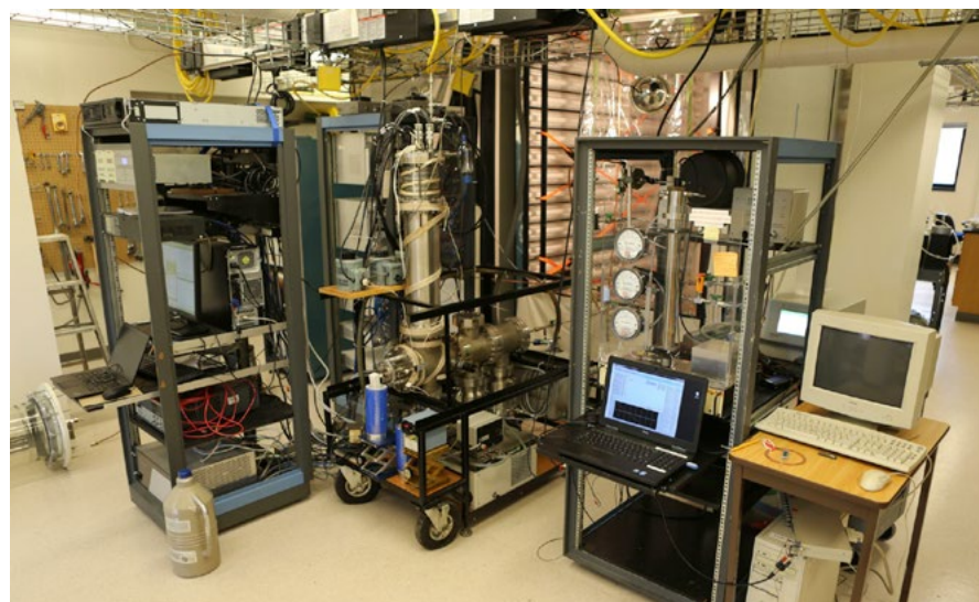
Environmental chamber and analytical instruments used to investigate the formation and chemistry of secondary organic aerosol particles under simulated atmospheric conditions. David Oonk/CIRES
