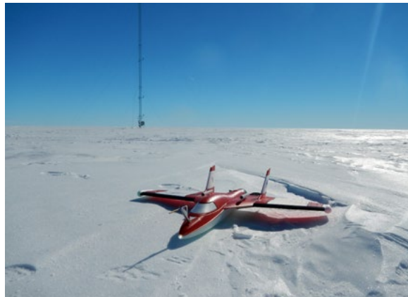
SUMO UAS and a 30-m tall tower automatic weather station on the Ross Ice Shelf, Antarctica.
