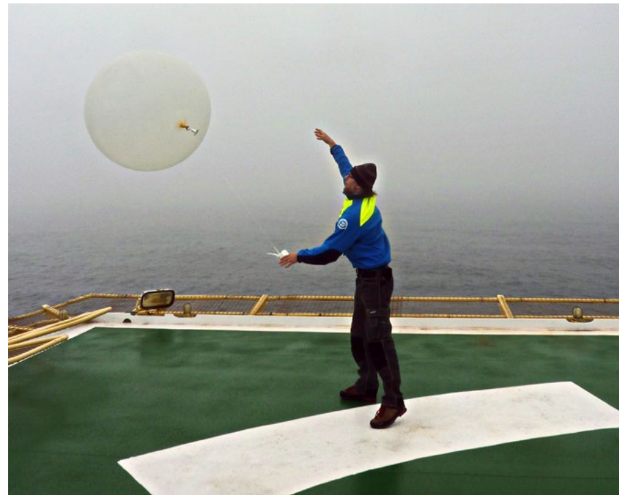
CIRES scientist Matthew Shupe launches a radiosonde from the deck of icebreaker Oden during the Arctic Clouds in Summer Experiment (ACSE) in summer 2014. Michael
