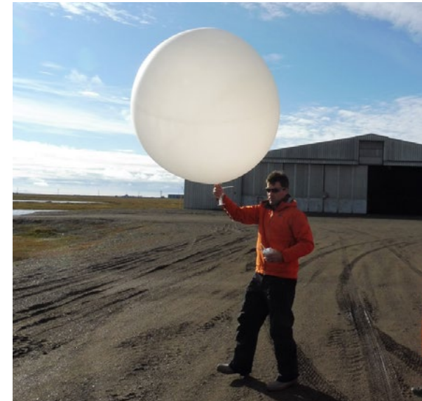
Gijs de Boer releases a ballonsonde while on an atmospheric science mission on Alaska's North Slope.
