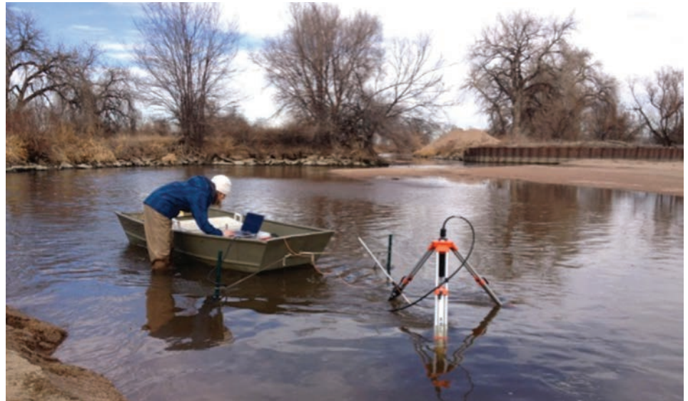
Above: Lindsay Chipman, Ph.D., deploys her Acoustic Doppler Velocimeter. Photo credit: Tommy Detmer
