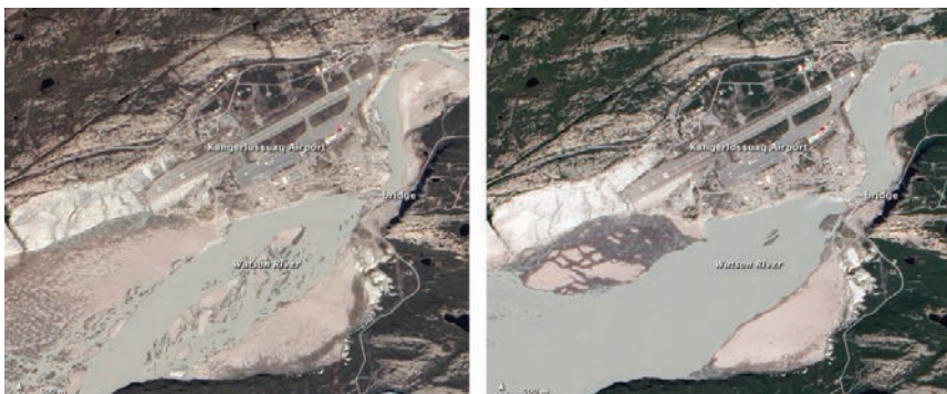
Although the Greenland Ice Sheet undergoes seasonal melting each summer, surface melt during July 2012 reached record levels. Runoff from the ice sheet flooded the Watson River and swept away parts of a bridge in the town of Kangerlussuaq. The left image is from May 31, 2012, prior to the melt. The right image is from July 25, 2012, after the record surface melt.
