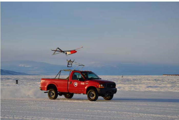
An Aerosonde unmanned aerial vehicle being launched from the top of a pickup truck at the Pegasus ice runway, McMurdo Station, Antarctica, in September 2012. Photo credit: John Cassano
