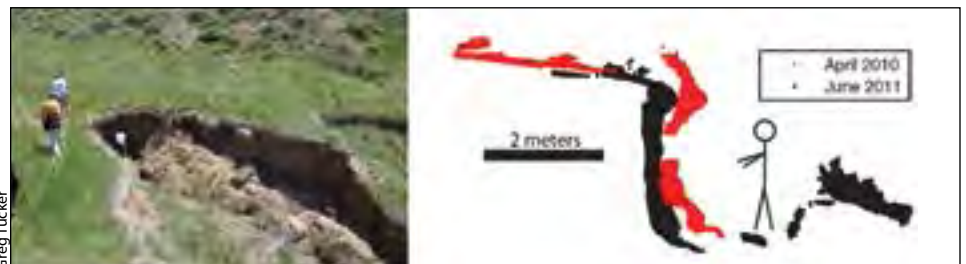
Left: A typical gully head near the West Bijou Escarpment. Right: Cross-sections of the gully head obtained with a ground-based laser scanner, showing morphologic change over a 14-month period
