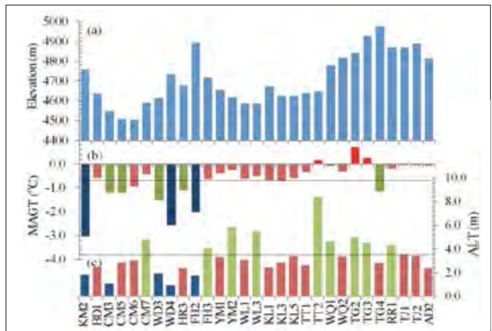
Figure 1: (a) Site elevation; (b) mean annual ground temperature (MAGT) at depth of zero amplitude; and (c) active layer thickness (ALT) along the Qinghai-Xizang (Tibet) Railroad.
