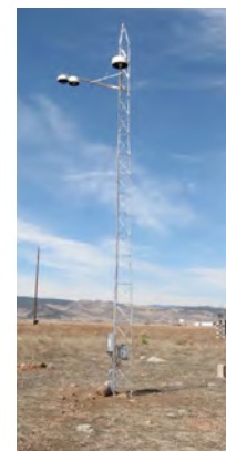
View of the albedo tower located at Table Mountain, approximately 10 miles north of Boulder, Colo. Mounted on the tower is the head of an MFRSR. Other instruments are radiometers measuring reflected UV-B and reflected Photosynthetically Active Radiation (PAR).
