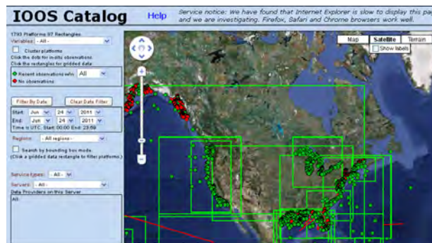
Figure 1: The Integrated Ocean Observing System (IOOS) Catalog uses ISO metadata and Open Geospatial Consortium (OGC) services to provide a centralized gateway for the discovery of ocean observation-based data sets.
