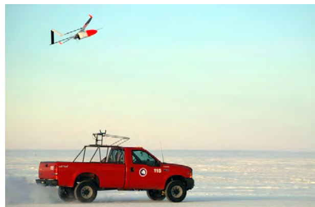
Aerosonde UAS being launched from the roof of a pickup truck at the Pegasus white ice runway, Antarctica.
