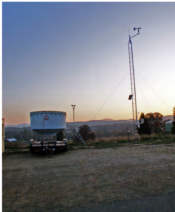
NOAA instrumentation at the Mariposa airport during sunset. From left to right, the photo shows a vertically pointing S-band (2.8 GHz) profiling radar, a Parsivel disdrometer and an anemometer mounted on a 10-m tower.
