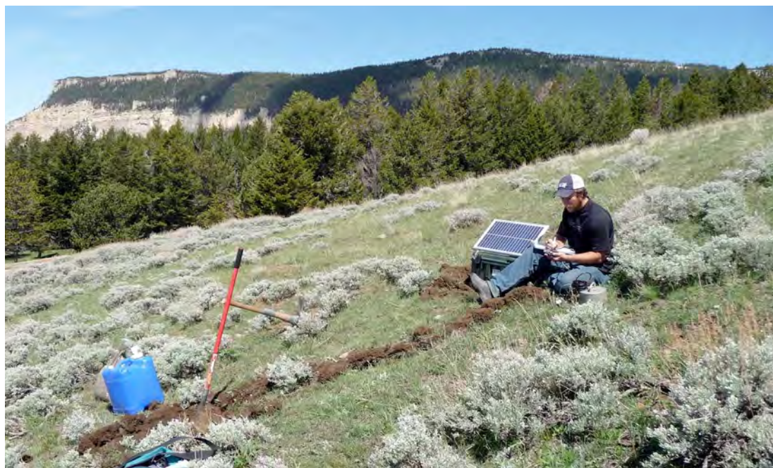
CIRES undergraduate assistant Jeremiah Silver installs a short period seismometer in Bighorn Mountains, Wyo.
