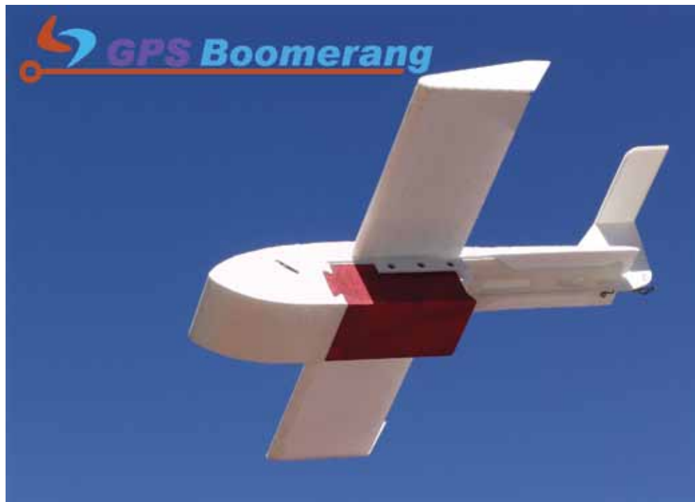
Figure 2: The mini-glider was developed in New Zealand and is being modified at CIRES to provide onboard archiving of temperature, humidity, pressure, wind speed and direction, and GPS flight coordinates.
