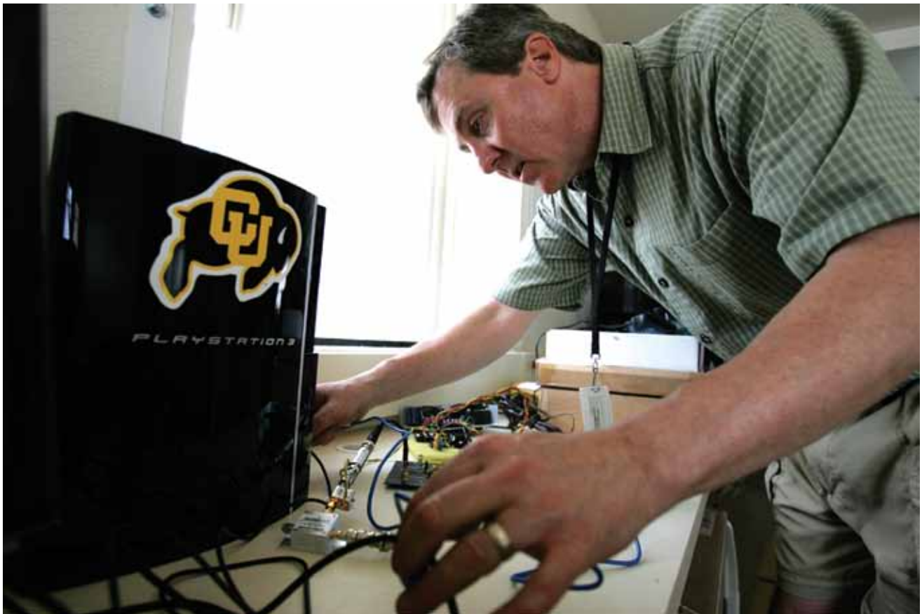
Christopher Williams works on the prototype of his less expensive vertical-profiling radar. The system uses a Sony PlayStation to process inputs from a set of three $200 radar dishes.
