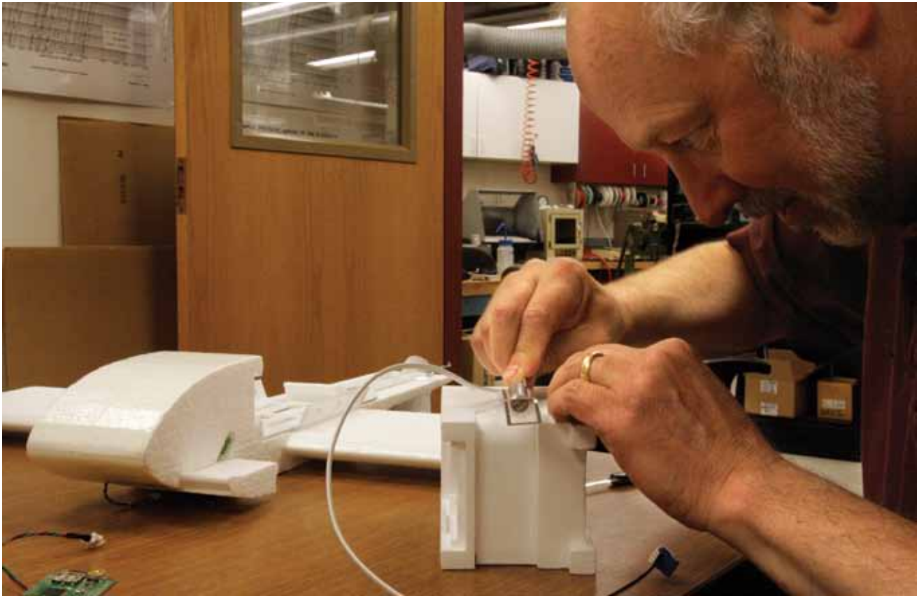
Don David begins mounting a radiosonde to a DataBird glider, for testing.
