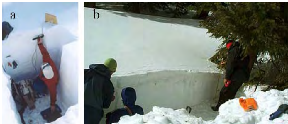
Figure 1. (a) Snow grain size stratigraphy measured at 2 cm sampling interval using the ASD-FR, Red Mountain Pass, CO. (b) Excavated snow trench extending radially from a coniferous tree trunk, Wolf Creek Pass, CO. - note the increase in snow depth with distance from the tree.
